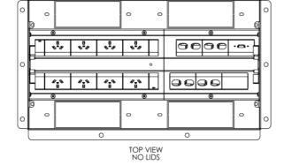
**STEP 3:** FIT BRACKET TO PERFORATIONS ON UNDERSIDES AND FIT BOX TO TOP
