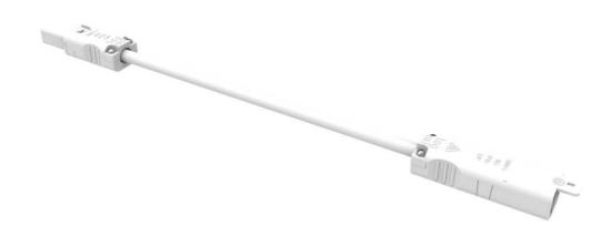
Ordinary duty leads are used for power distribution within furniture. Interconnecting cables are manufactured from 3 core 1.5sqmm flexible cable. They are rated at 16amp and are terminated with new male and female 'CMS' BS EN 6135:2009 compliant connectors Interconnecting cables are available in standard lengths from 1000mm, in 1000mm increments.
