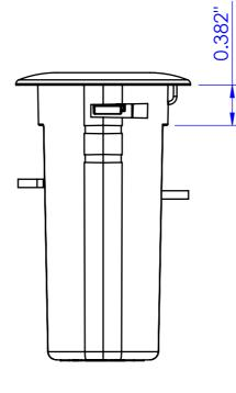
MIN TABLE THICKNESS: 0.5" MAX TABLE THICKNESS: 1.5"
