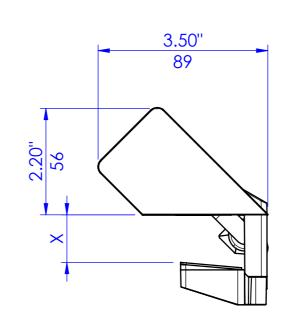
MIN TABLE THICKNESS: 0.75" (19mm) MAX TABLE THICKNESS: 1.25" (32mm)
