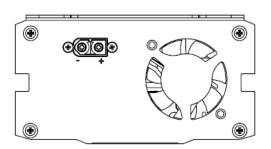
2. Connect the XT60 DC IN via XT60 interconnecting leads to DC OUT 1 on the docking station (FR210DS).
