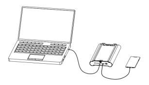
The power bank (FR210PB) can recharge any USB C or USB A compatible device(s). Simply plug in the device and the power bank will auto detect that a device has been plugged in and power on. Four white LED's will illuminate to indicate the power bank's charge level.
