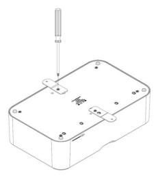
2. Rotate the fixing bracket outwards, the small metal tab on the bracket will align/fix into the outward position hole. This secures that fixing bracket so that it won't rotate once screwed into place.
