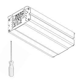
Position and screw Inverter (FR210I) into place on the underside of the workstation using 4qty 6G screw (or screw of your choosing). There are 2 screw fixing locations at each end of the inverter.
