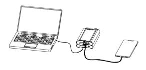
The power bank (FR210PB) on top will become the master unit. The charge level will be displayed via the 4 LED's on the master unit. The second Power Bank will become the slave unit.
