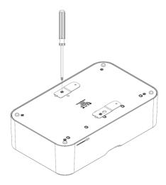
1. When first unboxing the Charging Station (FR210CS), the fixing brackets will be secured in the folded in position. Loosen the screw that secures the fixing bracket in place. Note that the screw will need to be lose/removed so that the small metal tab on the fixing bracket is able to clear the hole that's securing it in place.
