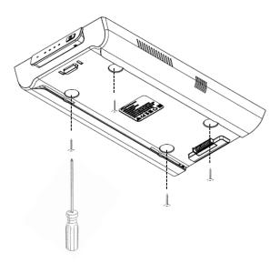
Position and screw the Docking Station (FR210DS) into place on the underside of the workstation using 4qty 6G screws (up to 8G will fit). There are 4 screw fixing locations on the underside of the Docking Station.
