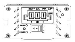
Connect the AC out via the TAG Panel Mount at the front of the inverter. Using CMS TAG soft wiring your able to easily connect to CMS products such as SW1804 (inline 4 GPO outlets).
